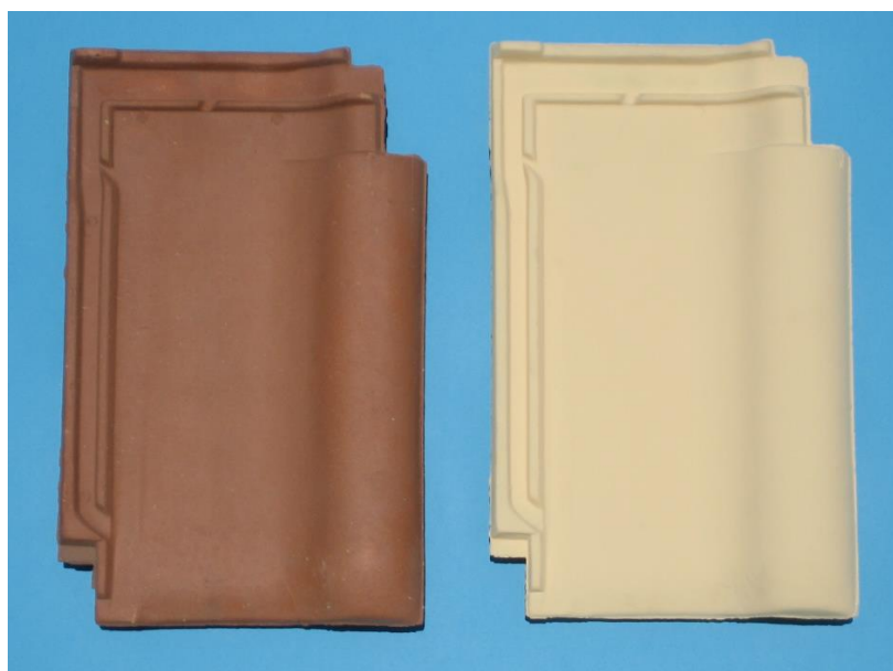
Figure 9. Crude red-brick ( \beta_s = 0.53 ) and painted one (bright brown, \beta_s = 0.30 )
