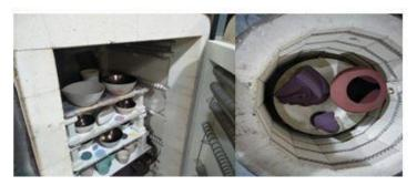
Fig7. Glossy firing with electric kiln at pre-testing stage
