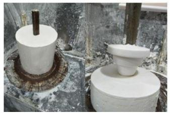
Fig4. Jiggering plaster models
