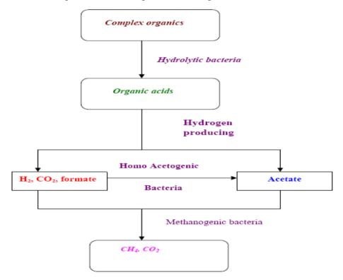
Figure 3. Biogas production process (Omer, 2003).
