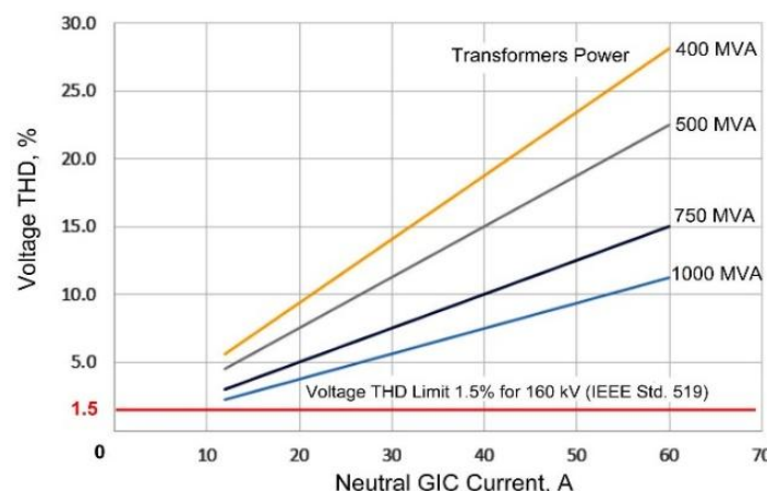
Figure4. Total harmonic distortion (THD) generated by a transformer into a high-voltage circuit as a function of GIC value in the neutral conductor [9]. The maximum permissible value of THD for 160 kV overhead power transmission lines is 1.5% [10].
