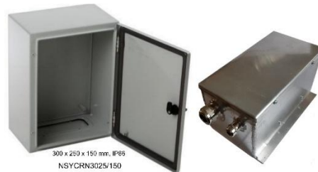
Figure9. Sealed aluminum container (right) used for protective electronic relay installation near or power transformer. Another possible option - small standard metal enclosure (left) NSYCRN3025/150 type produced by Schneider Electric.
