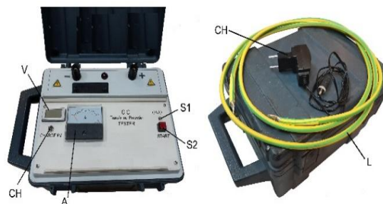
Figure10. Portable tester for testing the GIC protective relay serviceability designed and constructed by the author.
