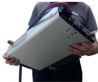
Figure6. ADC7480 battery charger with output voltage of 0 – 300 V and output current up to 14A.
