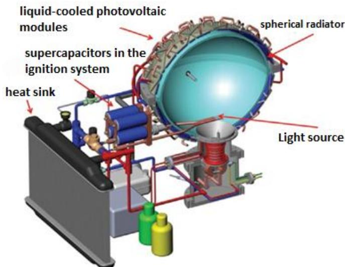
**Figure7.** SunCell device diagram ("solar cell")
