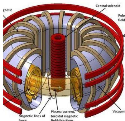
**Figure 5.** Closed plasma trap (tokamak).
