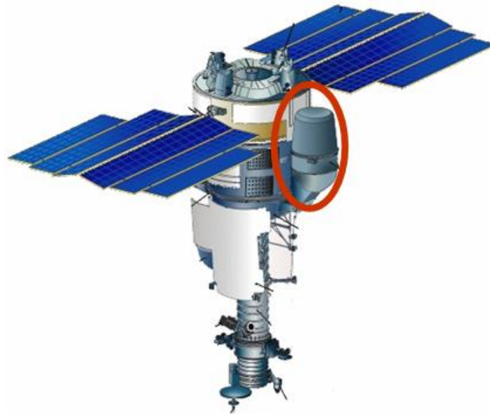
Figure1. “PAMELA” in a container on the Resurs-DK satellite
